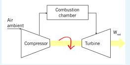
Combustion turbines are constant-volume engines and their power output is directly proportional to the air mass flow rate entering the engine.
