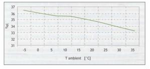
A cogeneration plant located near Turin (Italy), a generating set composed of an engine coupled to an alternator has been cooled using Breezair evaporative cooling. In this plant the heat generated by the engine combustion process is conveyed and used to produce heat in the form of carriers including hot water or steam for various civil and industrial uses. The cogeneration plant has a power production rating of 2 MW and hot water production of 90m<sup>3</sup>/h.
